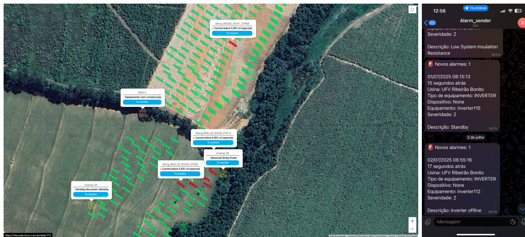
Figure 5: Georeferencing with alarms and notifications on Telegram.
